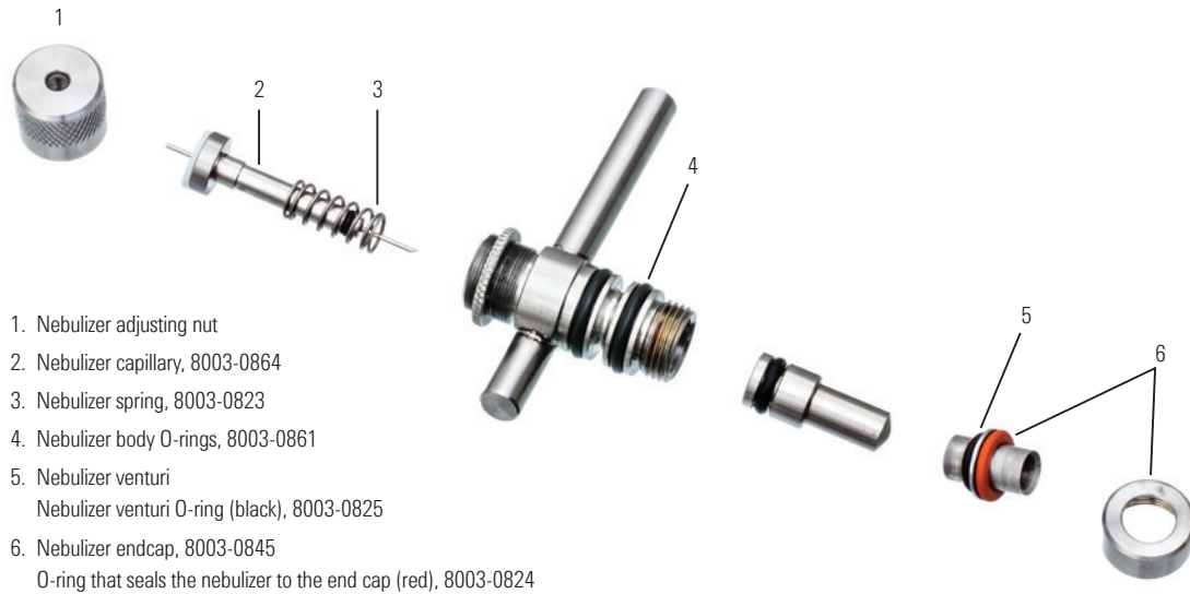
Exploded view of Nebulizer assembly, 8003-0828
